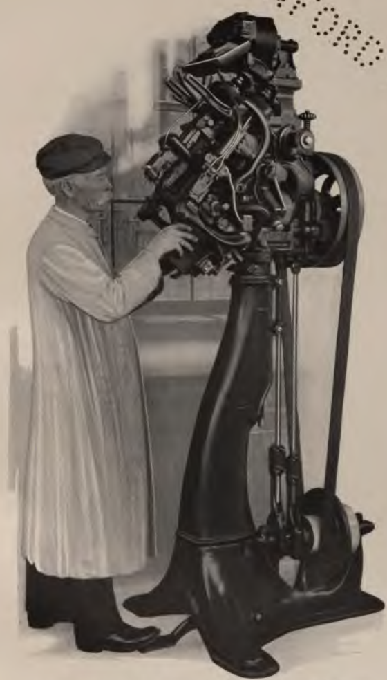
Operating the Rex Pulling Over Machine
